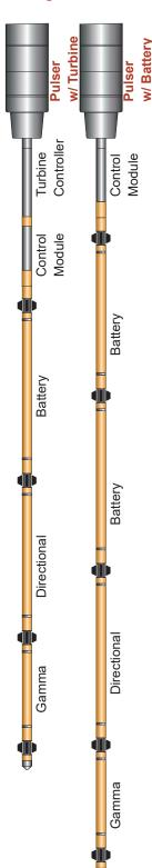
The Top Mount Pulser is an upgrade option that offers all the benefits of top mount architecture while maintaining the reliability and flexibility which is required in today's market. The assembly is a drop in replacement for any of the standard Tensor Elite Pulsers.
