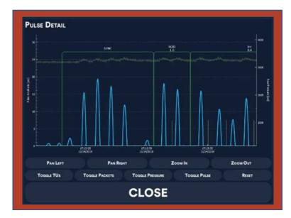
Next Generation MWD Compatible System provides exceptional single or dual transducer pressure pulse decoding.
